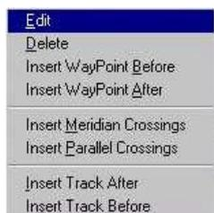
A new track can be created by opening a new file in the file menu. After selecting a geodetic datum and adding a required waypoint the next waypoint can be added after pressing the add button. The new track or area can be saved by pressing the finish button. Track files must be saved as \*.trk file and area files as \*.are file.
